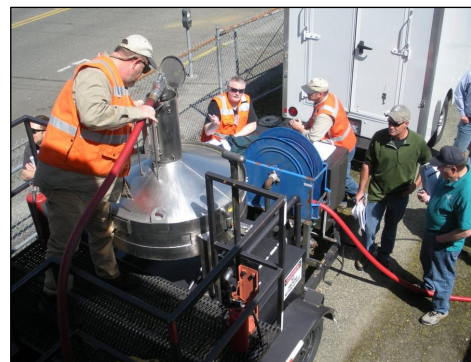
Weights and Measures Inspection of a Home Heating Fuel Delivery Meter NIST Photo
